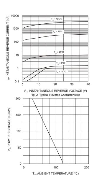
Fig. 4 Power Derating Curve, Total Package
